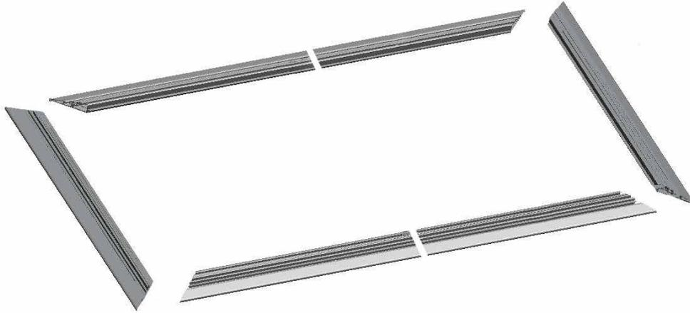
**Step 3.** Insert the *Center Joint (e)* connectors into one-half of the horizontal frame and secure with two screws. Once secure, connect the other half of the horizontal frame and fasten with two screws. **NOTE: Make sure to insert 3 brackets (g) on each of the horizontal frames (Top and bottom) after connecting the center joints.**
