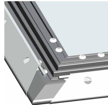
**Step 5.** Starting from all four corners, hook the *Springs (a)* through the hole located on the screen material's outer edge. First, hook the small spring head to the frame. Then using the *Spring hook (b)*, hook the other side of the spring to the material. **NOTE: Only do the corners for this step.**
