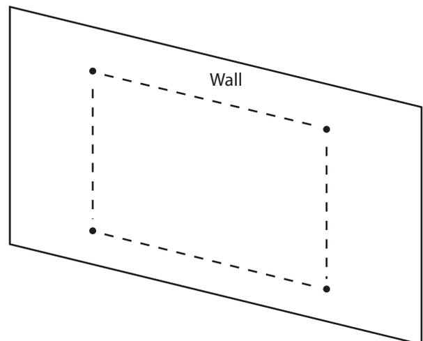
**Step 3.** Place the wall *anchor (f)* followed by an *M5x40 screw (j)* to the wall for each bracket on the frame. Next, using two people, carefully position the screen onto the wall. Your installation is now complete.
