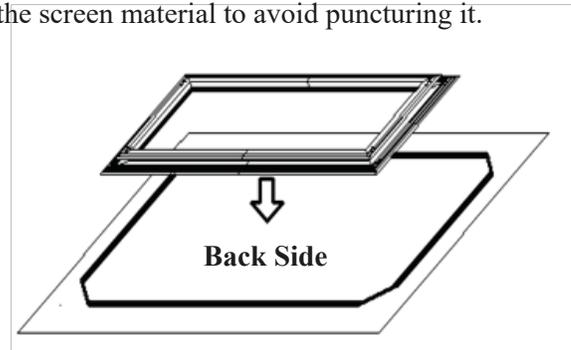
**Step 3.** Insert the four horizontal and two vertical *Tension Rods (i)* into the corresponding sides of the screen material, while keeping the material laying flat. Careful not to snag on the holes at the edge of the material during this process; forcing the rods may damage the screen material.
